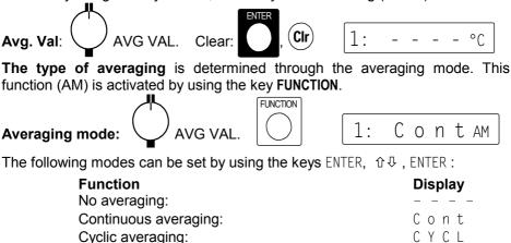
For **averaging single measurements** the averaging mode 'Cont' must be selected, measuring and print cycle must be cleared and the key **MANUAL** must be pressed each time. In function AVERAGE the average value is indicated and can be printed at any time by using the key **OUTPUT** (see 8.3).
