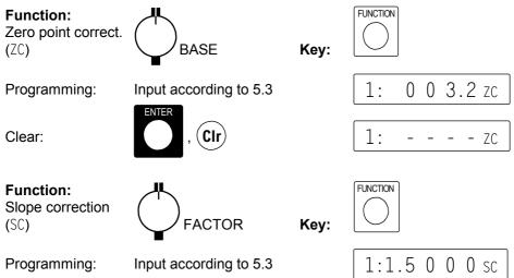
If correction values are programmed and, as a result, the measured value is corrected, the arrow **CORR** will be indicated in the display.
